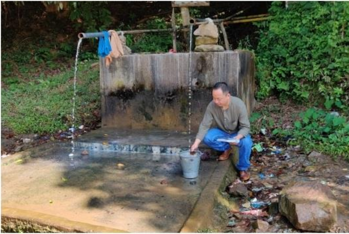
Spring discharge measurement during Post-Monsoon and pre-monsoon
