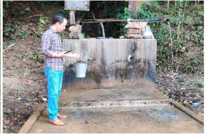
Spring discharge measurement during Post-Monsoon and pre-monsoon
